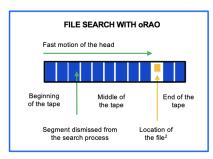
Improve file access and recall times with IBM LTO 9 tape drive
